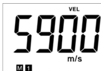
Last applied sound velocity & unit no.
