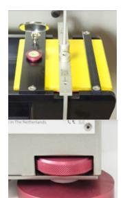
The spirit level is located on the test specimen. Once leveled further calibration is not required.
