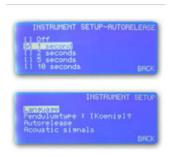
The Pendulum hardness tester is suitable for both Persoz and König Tests. Switching between the methods only takes a push of a button.
