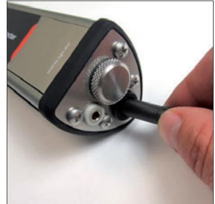
The other side of the earth cable is plugged into the supplied crocodile clip (D). This crocodile clip must be connected. When used on an untreated piece of the substrate
