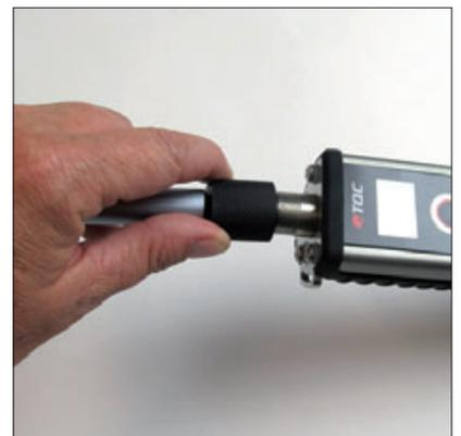
The grounding cable (C) must be inserted into the black bus (I) be on the bottom of the device. (near the battery compartment)
