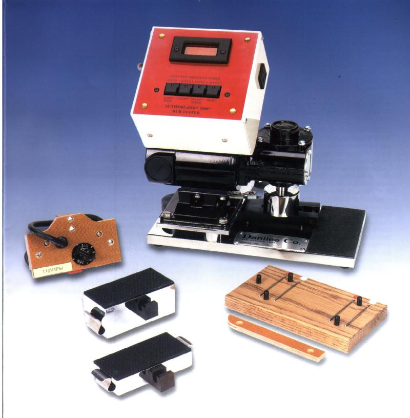
Illustrated is the 4-speed SUTHERLAND® 2000™ Rub Tester showing two-pound and four-pound weights to which test specimens are attached, the scoring device,
