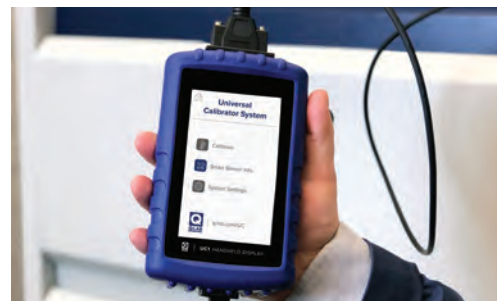
Calibrating your Q-SUN tester's irradiance and temperature is simple using the Universal Calibrator system.
