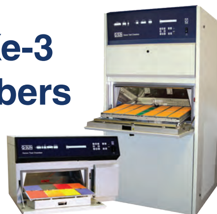
Q-SUN models range from an entry level, bench-top model to a full-featured tester with humidity control, water spray, and chiller.
