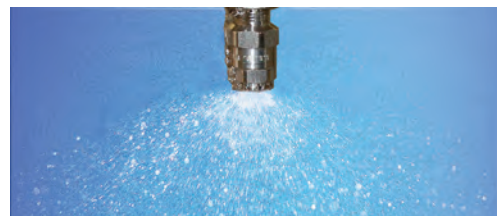
Outdoor moisture attack is simulated by spraying pure water onto specimens.
