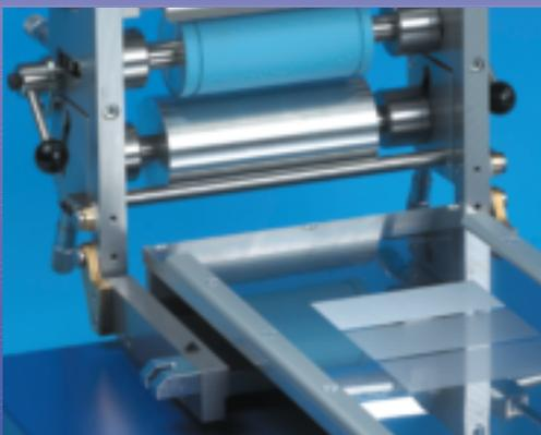
High quality proofs using gravure, gravure-offset or flexo inks are produced instantly using the K Printing Proofer. Featuring electronically engraved printing plates and variable printing speeds of up to 40m/min, this is an essential tool for all those involved in the manufacturing or use of liquid inks. Ideal for R & D and computer colour matching data, quality control and presentation samples. The K Printing Proofer is very easy to clean and all parts are solvent resistant.
