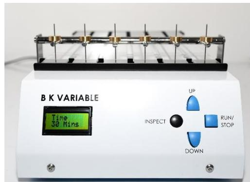
Use the recorder on a firm bench and do not restrict ventilation by using in a confined area. Any surplus paint should be wiped off the recorder with a dry cloth. We do not recommend the use of solvents.
